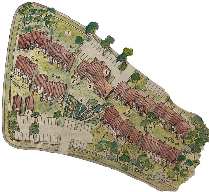
Figure 3.5. Schematic site design for Muir Commons Co-housing: 1.common house, 2.terrace, 3.tot lot, 4.garden, 5.gathering nodes, 6.wood and auto shop, 7.orchard. (McCamant & Durrett, 1994)
